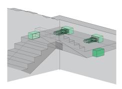
The impact sound insulation element SINTON® X decouples stair landings from masonry or concrete walls. SINTON® X consists of a polyurethane box with integrated elastomeric bearings for transferring loads, a filler for stabilisation during casting and a frame for fastening to the formwork. It is the basis for all other SINTON® X variants. Different forces can be transmitted depending on how the thrust bearings are placed.
